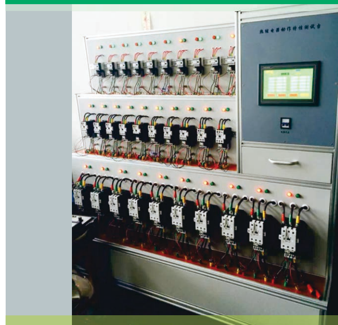
热继电器动作特性测试台 Thermal Relay Action Characteristics Test Bench
