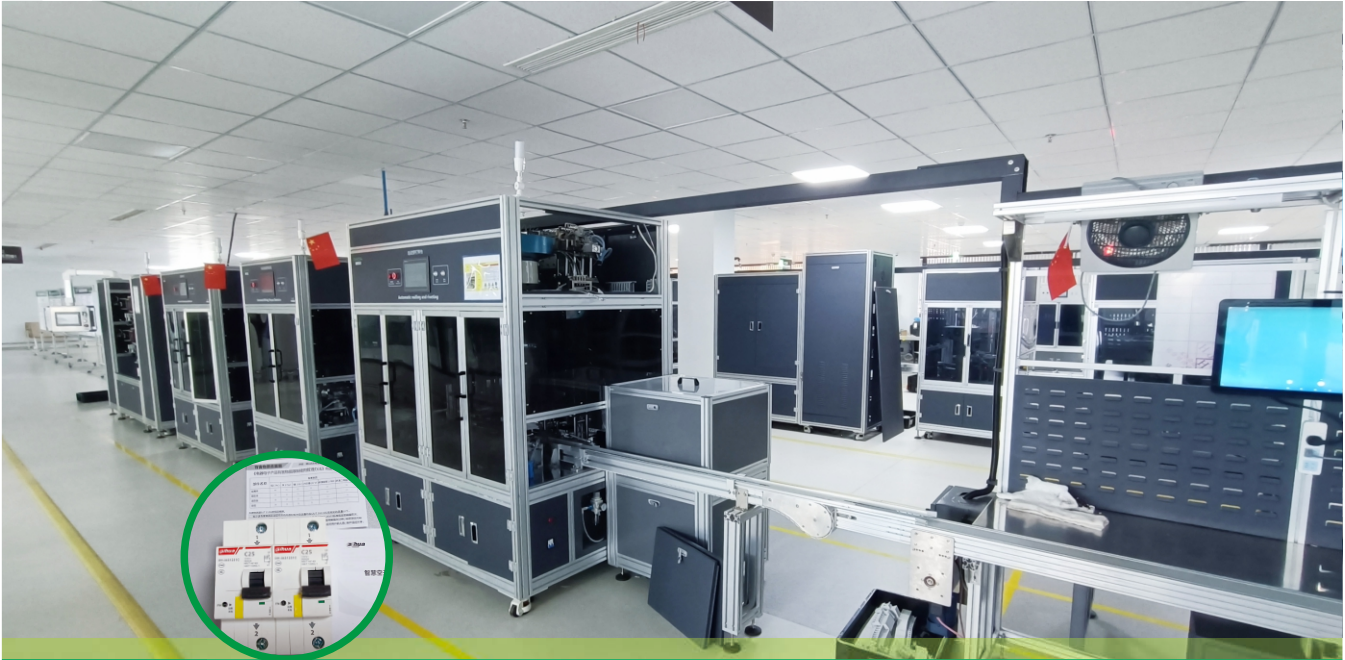
智能断路器（重合闸）前段调试检测线 Intelligent Circuit Breaker (Recloser) Front Section Debug Detection Line
