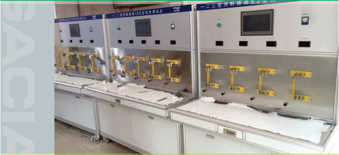
MCCB延时动作特性测试台 MCCB Delayed Action Characteristics Test Bench
