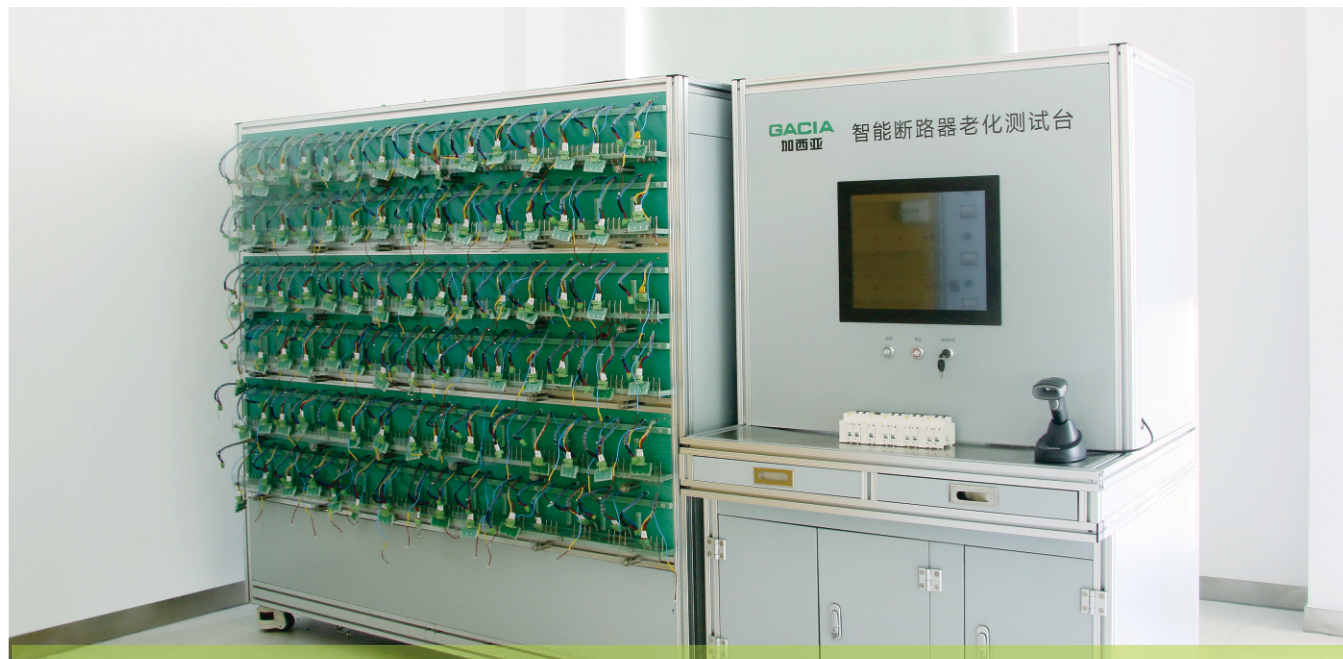
智能断路器老化测试台 Aging Test Bench for Small Leakage Circuit Breakers
