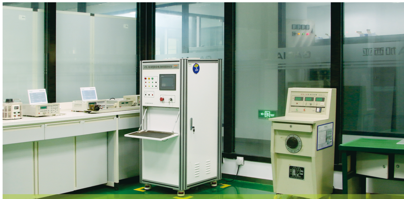
介电、冲击和B型漏电测试台 Dielectric, Shock and Type B Leakage Test Stands
