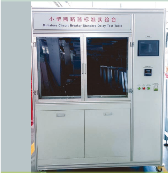
MCB长延时特性校验台 MCB Long-delay Characteristic Check Bench
