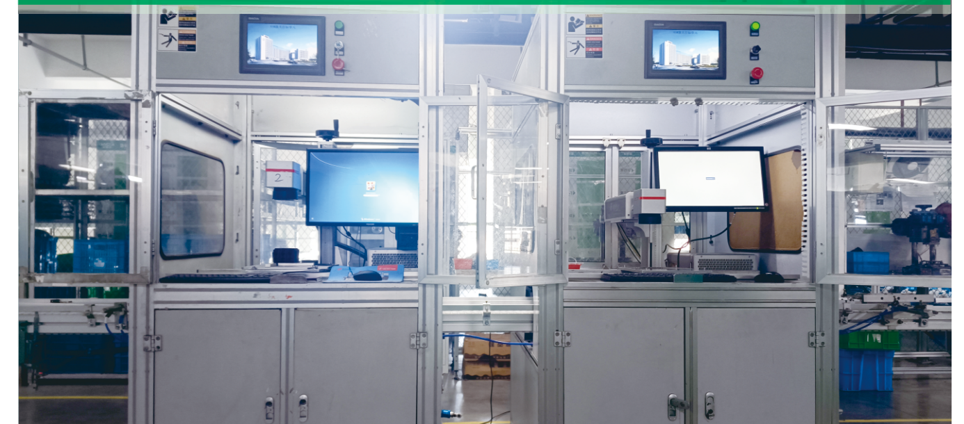
紫外线激光打码生产线 UV Laser Coding Production Line
