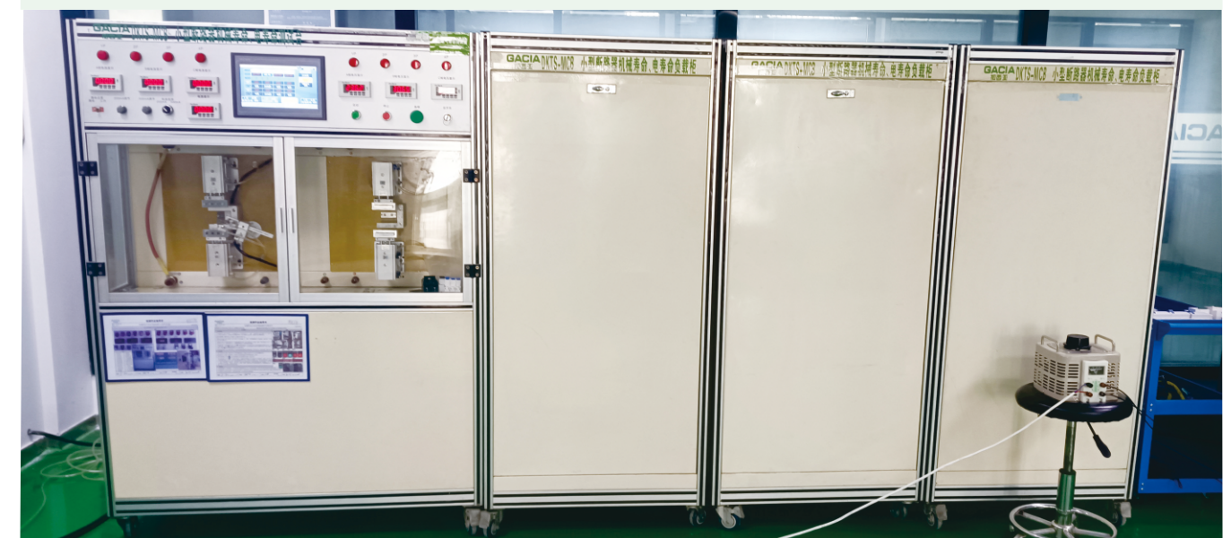
机械寿命、电寿命综合测试台 Mechanical Life, Electrical Life Comprehensive Test Bench
