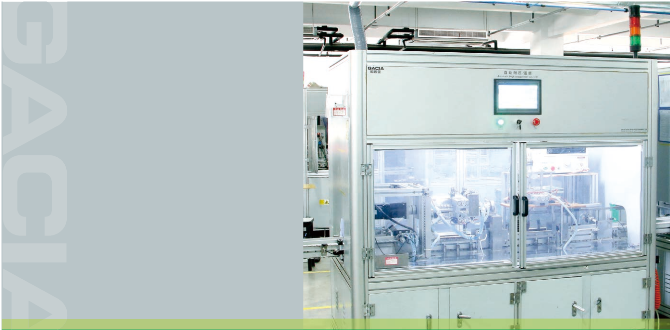
小型断路器通断、耐压特性检测单元 MCB On-off and Stand Voltage Detection Unit
