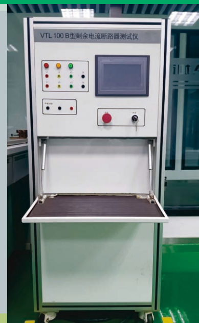
B型剩余电流测试台 Type B Residual Current Test Bench
