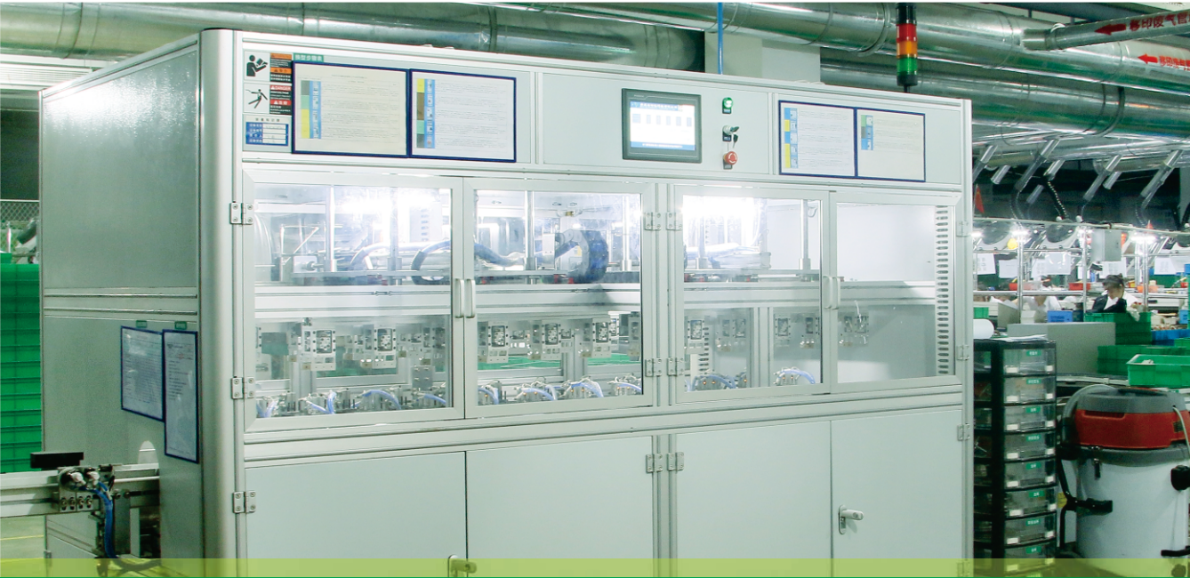
漏电断路器剩余电流测试台 RCCB/RCBO Residual Current Test Bencher
