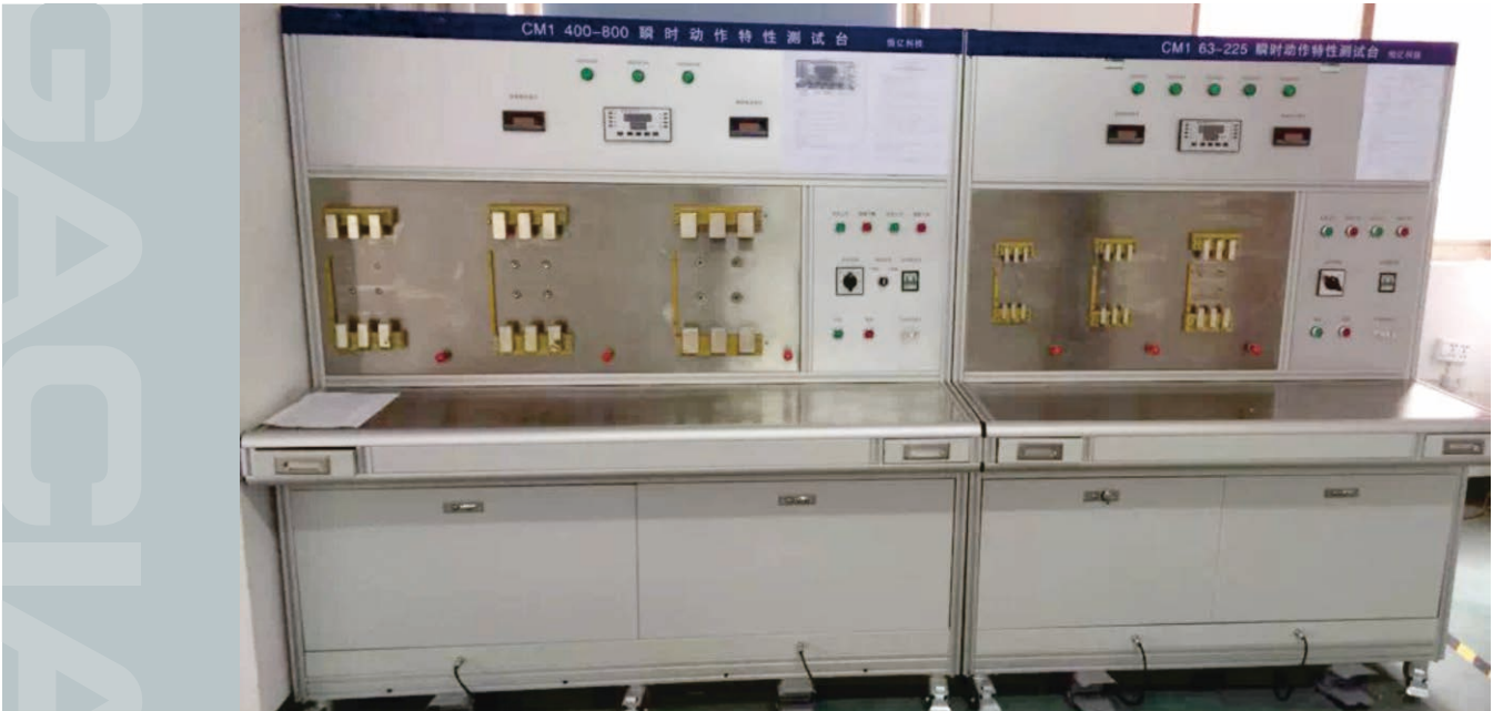
MCCB瞬时动作特性测试台 MCCB Instantaneous Action Characteristics Test Bench
