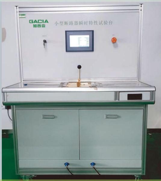
MCB人工瞬时校验台 MCB Instantaneous Calibration Bench
