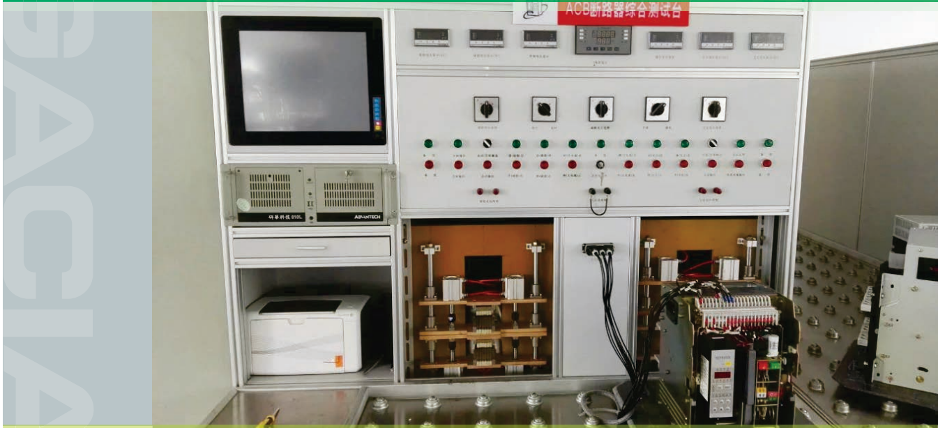
框架断路器综合测试台 Frame Circuit Breaker Integrated Test Bench
