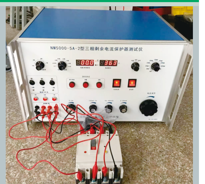
MCCB三相剩余电流保护器测试台 MCCB Three-phase Residual Current Protector Test Bench
