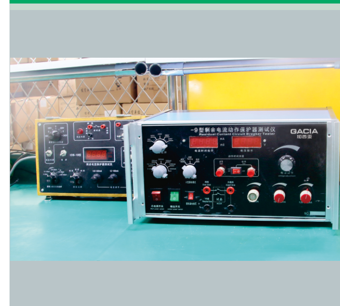
漏电剩余电流测试仪 RCCB Residual Current Protector Tester
