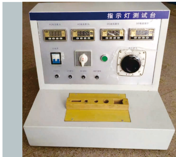
指示灯测试台 LED Test Bench
