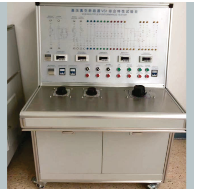
高压真空断路器综合测试台 High-pressure Vacuum Circuit Breaker Integrated Test Bench
