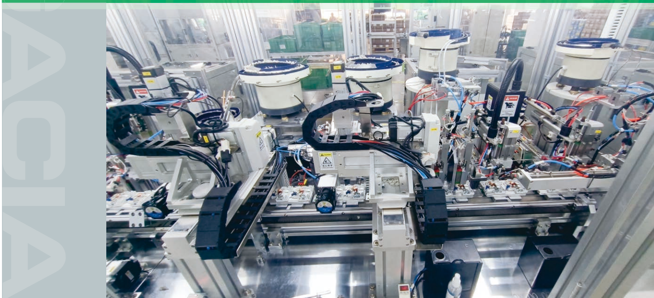
MCB自动组装跳扣、锁扣 MCB Automatically Assembles Jumpers and Locking Clasps
