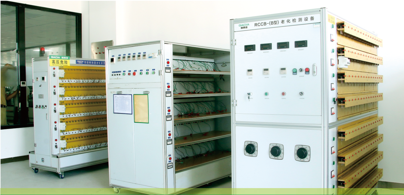
漏电断路器老化测试台 RCCB/RCBO Aging Test Bench
