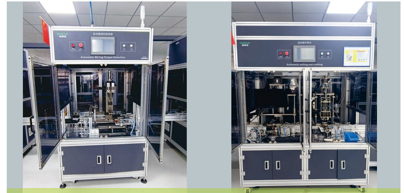
自动螺丝扭力检测单元 Automatic Screw Torque Detection Unit
