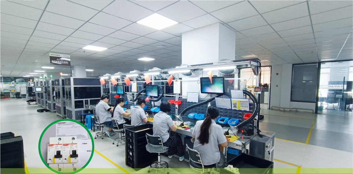
智能断路器（重合闸）后段调试检测线 Intelligent Circuit Breaker (Recloser) Rear Section Debug Detection Line
