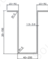
Fully Automatic Forming Channel Steel (U-shaped Steel) Small Edge: 20 - 40mm Web Height: 20 - 150mm Bottom Edge: 40 - 200mm Plate Thickness: 1.5 - 3.0 (0.3558); 3.5mm (02358)
